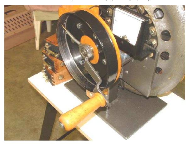
This Coil Tester was made from junk T parts and off the shelf parts from an industrial supply store. The cost including meter, stand and a new field coil was less than \$300.
