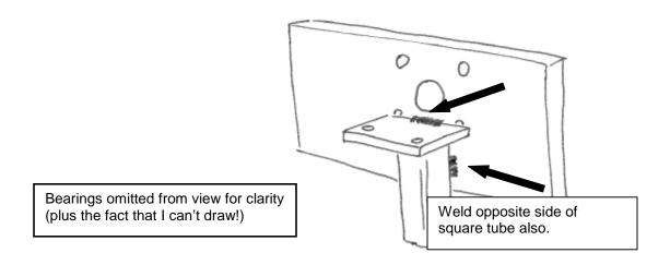
3. Position the welded up assembly onto the 8 X 12 inch base plate, centering left and right as shown. The front edge of the square tube should be set back 1 ¾ inches as shown. Weld around periphery as illustrated.
