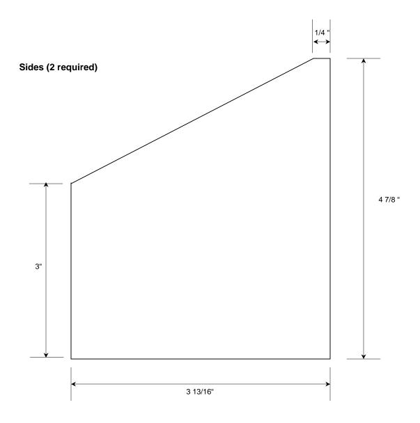
All coil box parts should be made of a stable hardwood such as Maple or Cherry. Use Baltic Birch plywood as a last resort. Plywood has a tendency to arc between the plys. Assemble using wood glue and finish nails. Give coilbox three coats of spar varnish to finish.
