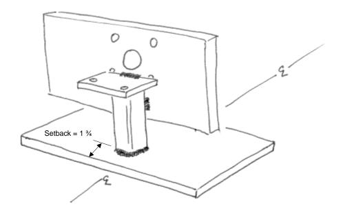
4. Add angle iron scrap as illustrated. This should be level across the top with the top plate. This item will be drilled later and the coil box added. Leave a gap between this scrap and the top plate as shown. Gap should be sufficient to allow wires to pass through, ¼ inch should be adequate.
