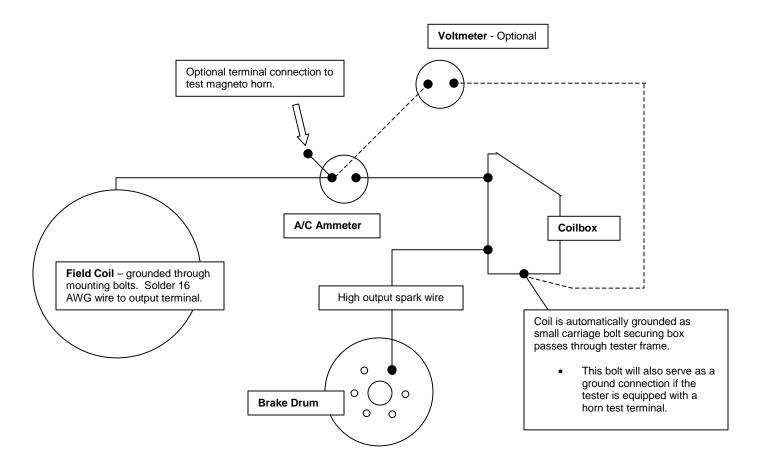
**Note**: All ground symbols eliminated to simplify wiring of tester. The coil box and field coil are grounded through their respective mounting bolts.
