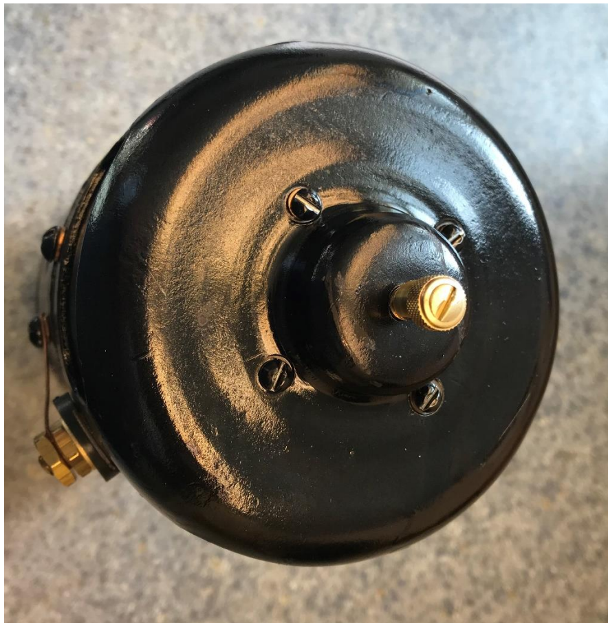
Figure 1. Generator Brush Cap Clamp Ring Screws
