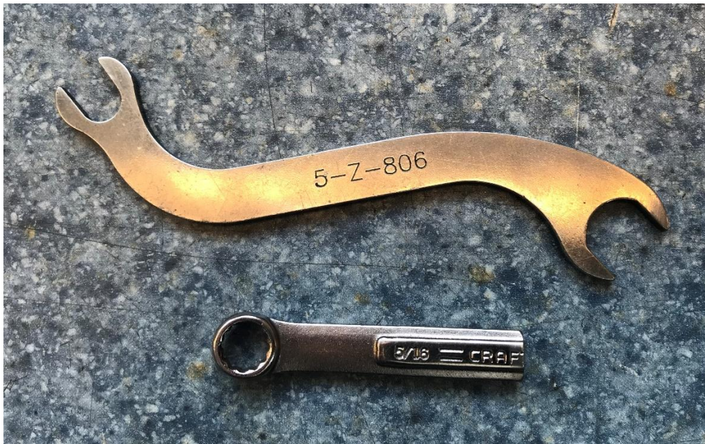
Figure 4 Special Third Brush Adjusting Wrenches.
