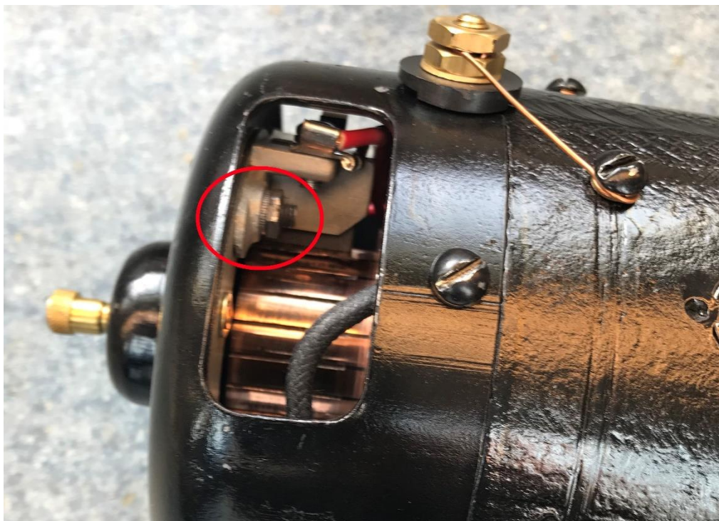
Figure 3 Third Brush Clamp Nut Location
