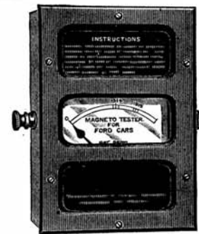
Fig. 91. Ford magneto tester. Note how the scale is marked. See text.
