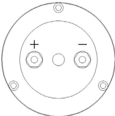
The polarity of the connections to the voltmeter is important and the (-) connection should always go to ground in a negative ground system. The (+) connection would connect to whatever point in the system that you wish to monitor.
