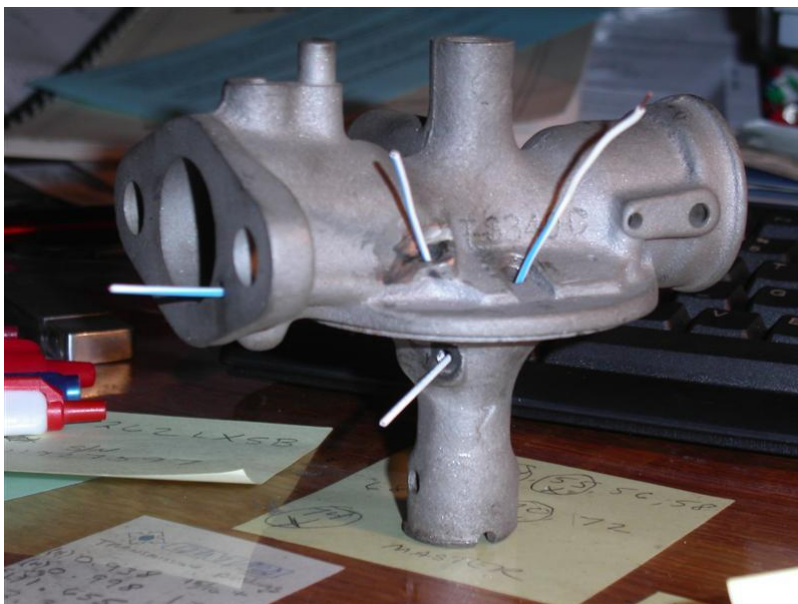
Carb shown with plugs removed and wire inserted to clean out passages.
