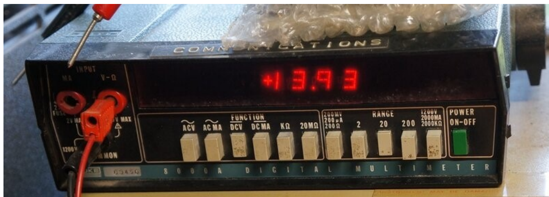
13.93V charge voltage into simulated load of a 60,000uF capacitor and 12V 5W lamp.
