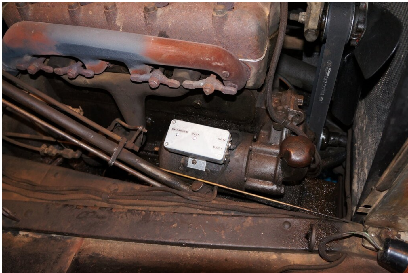
Homemade regulator uses comparator controlled grounding switch.
