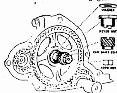
Driving Gear Mounted on Cam Shaft
