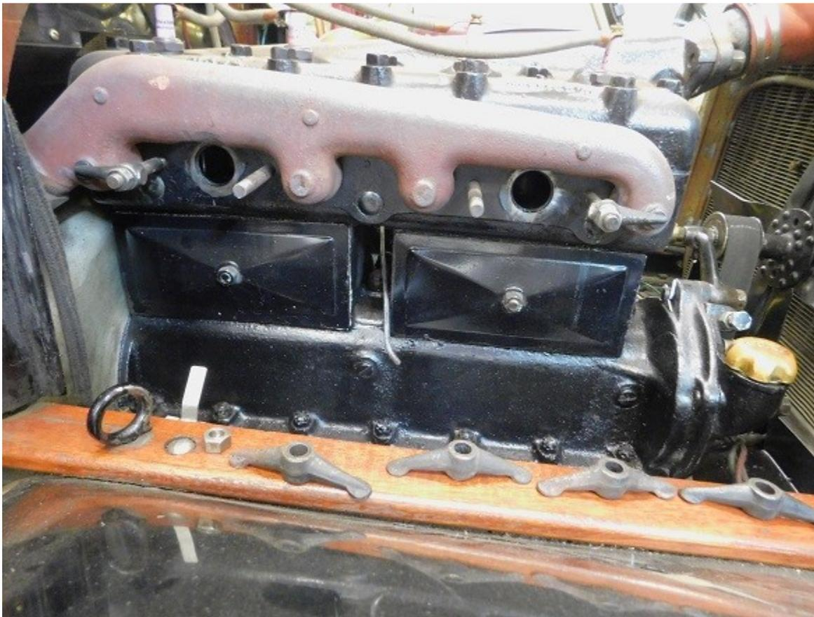
We removed the previous intake and carburetor, using half clamps to hold the exhaust manifold so we would not need to replace the four exhaust manifold glands. We cleaned the intake ports using a razor blade, scraping away traces of silicone sealant.
