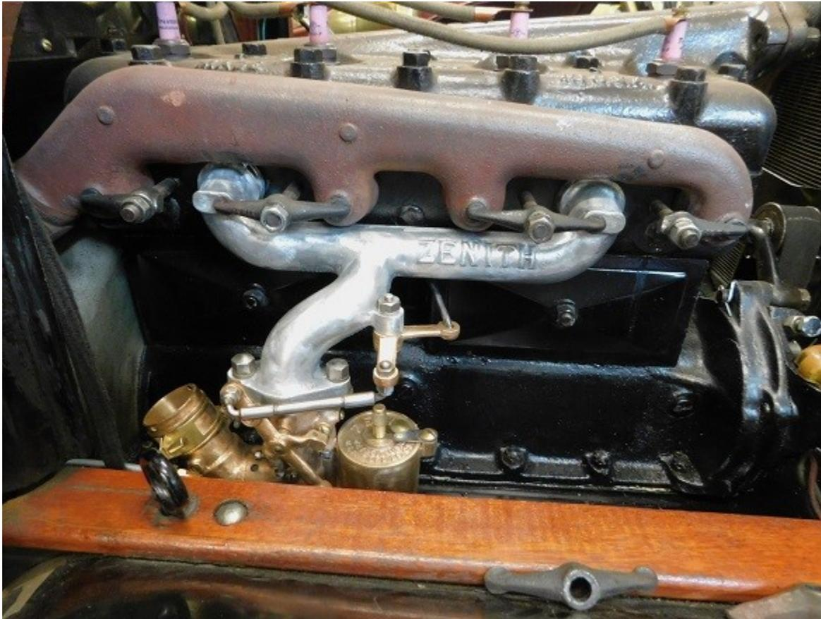
*The stock throttle rod was not quite long enough so we fabricated a new one using 4130 3/16" steel rod. 3/32" (#40 AWG) holes were drilled in each end for cotter pins.*
