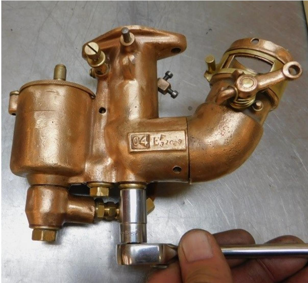
*We pulled the carburetor and drained the gas from it. The jet covers were removed so we could try another set of jets.*
