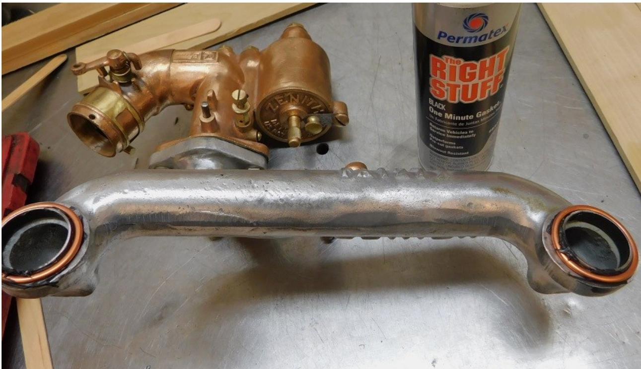
We put a tiny bead of "The Right Stuff" around each steel ring, then laid the glands on top, and put another
