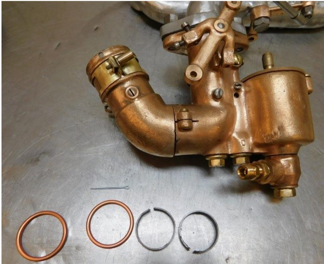
*With our manifold and carburetor rebuilt and ready to install we cleaned the steel rings from the previous intake. The copper gland rings are new.*
