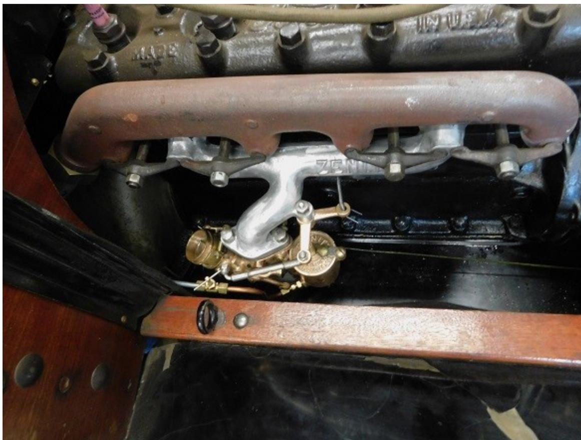
*With the carburetor installed we turned on the gas and checked for leaks. It had none so we are ready to go!*
