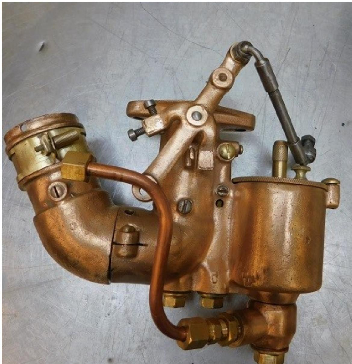
*We ended up removing the carburetor in order to be able to install and tighten the fuel line properly. Access is terrible with the carburetor installed.*
