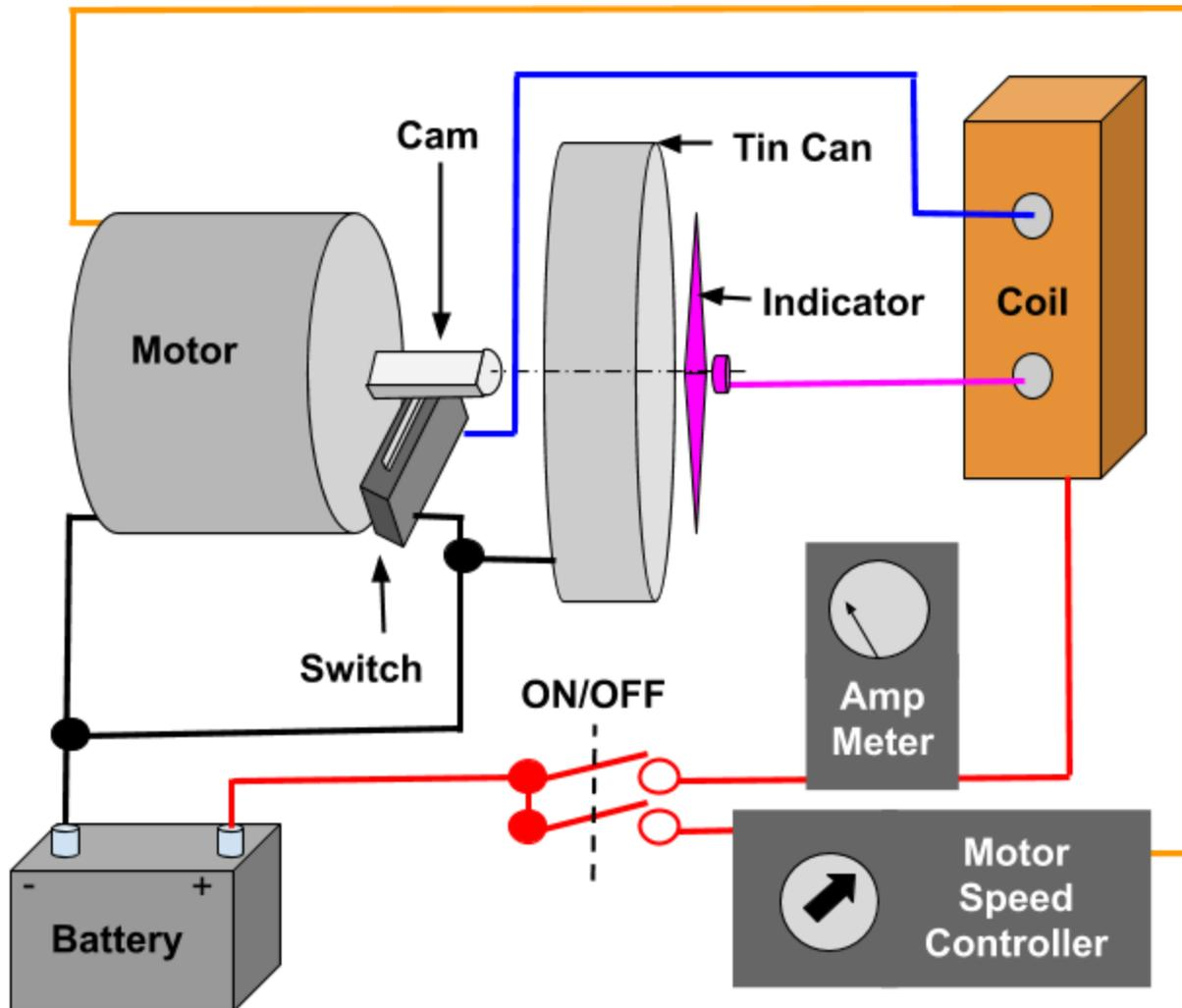
Simply put the MCCT is a Ford coil triggered by a switch. This switch is controlled by a cam on a motor. The motor speed controller adjusts motor speed that controls the switching time to the coil very much like a commutator does on the Model T. The indicator turns and can display the spark on a scale similar to a Hand Crank Coil Tester (HCCT). Additionally an amp meter is used to display the amount of current flowing to coil.
