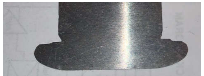
Figure 20. Clincher Profile Test Gage
