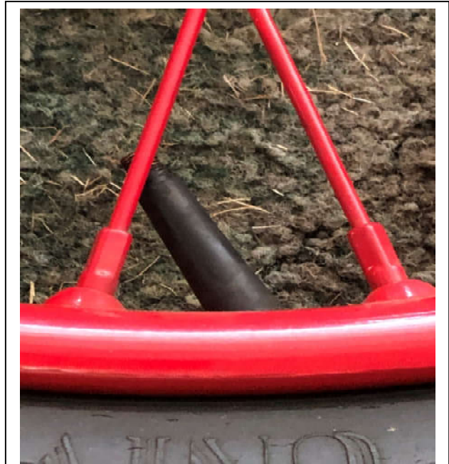
The Problem – Tire & Tube have shifted relative to the rim.
